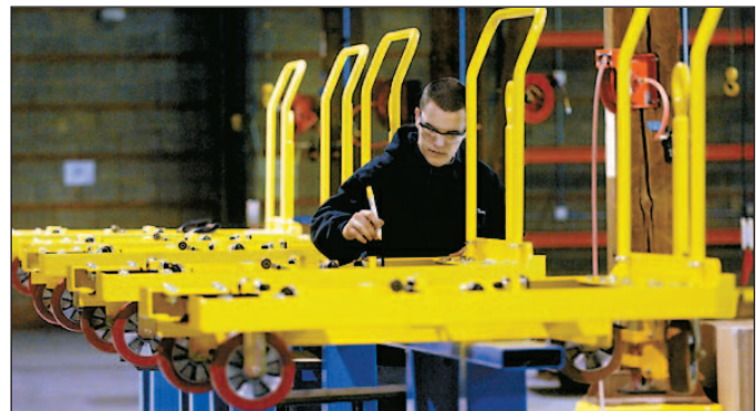
ABOVE: Paul Sibenik plasma-cuts a piece on a cart system for Lubrizol Corp. at Kinetic Technologies in Wickliffe. BELOW: Joe Lucas marks with paint bolts that have been set to a certain torque on carts at "K-Tec," which specializes in developing carts to replace forklifts.
